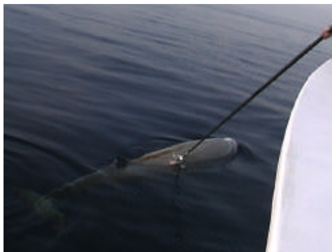
Fig. 5. Attaching a Dtag to a Cuvier's beaked whale using a hand-held pole. The tag stayed on for one full dive, and came off after the whale surfaced.
