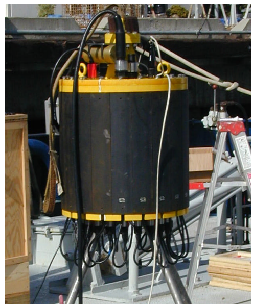
Fig. 1. IMAPS Integrated Marine mammal Monitoring and Protection System
