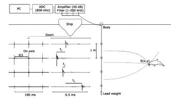
FIG. 1. Setup for recordings of *Tursiops aduncus*. The recording setup was similar for the *T. truncatus* recordings reported in the text.  $t_1$ ,  $t_2$ , and  $t_3$  are the time-of-arrival differences between the same click arriving on the four different hydrophones. [Jensen *et al.* (2009b), reprinted with permission from J. Exp. Biol.]
