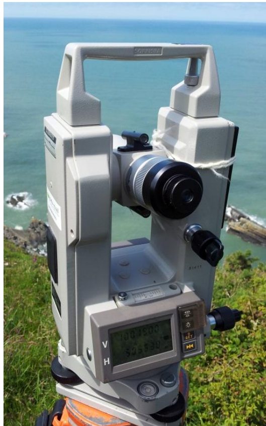
Figure 7. Digital Sokkia DT50 30x objective theodolite (Photograph - Tess Hudson)
