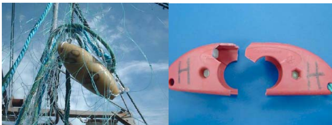
Figure 52: Pinger entangled in fishing gear (left), Durability of pingers is an issue (right)
