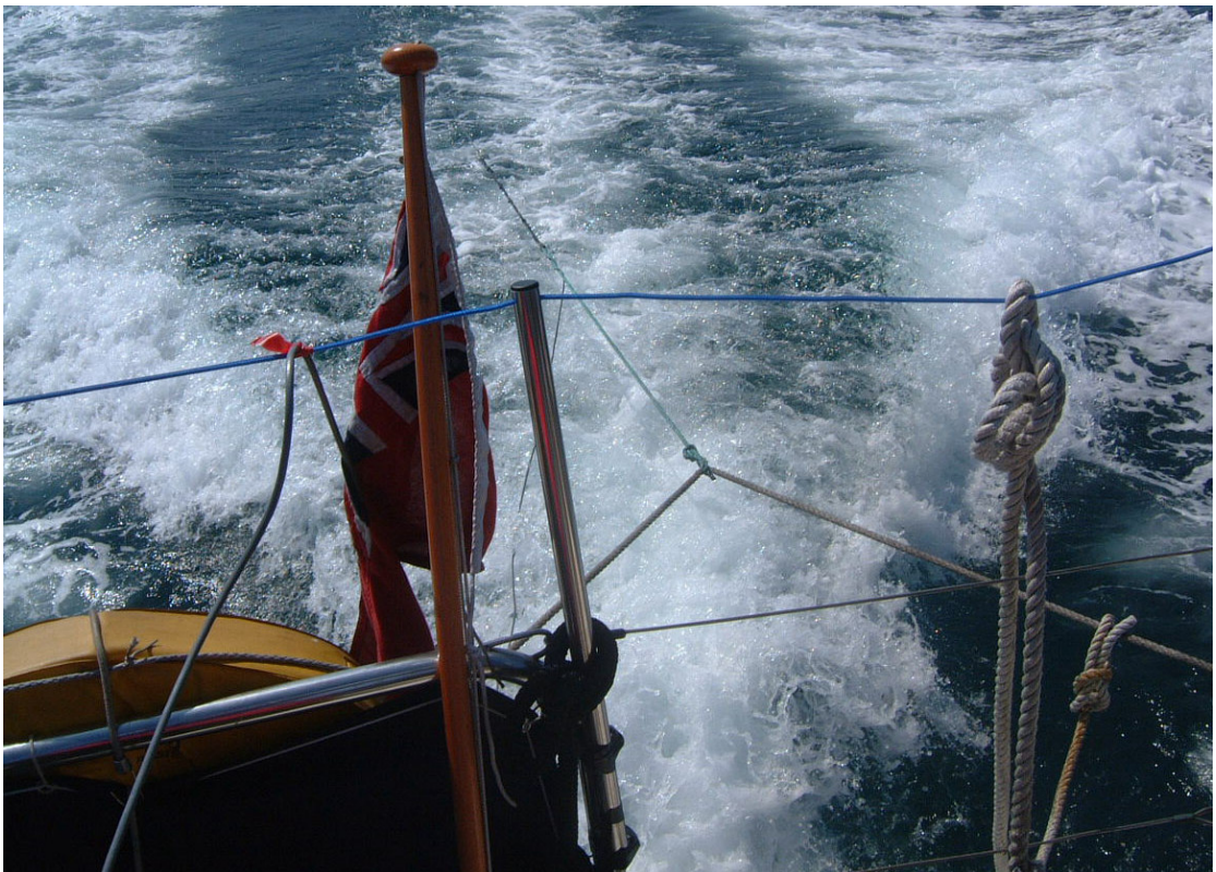
Figure 2. Photograph showing the fully deployed hydrophone, and central towrope attached to Liberty of Whites' port and starboard stern cleats.
