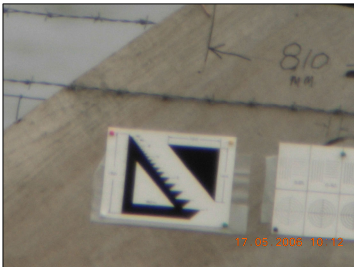
Figure 3.15: Images of the land based target taken with the digiscope at different stages of zoom. Images have not been cropped or transformed in any way.
