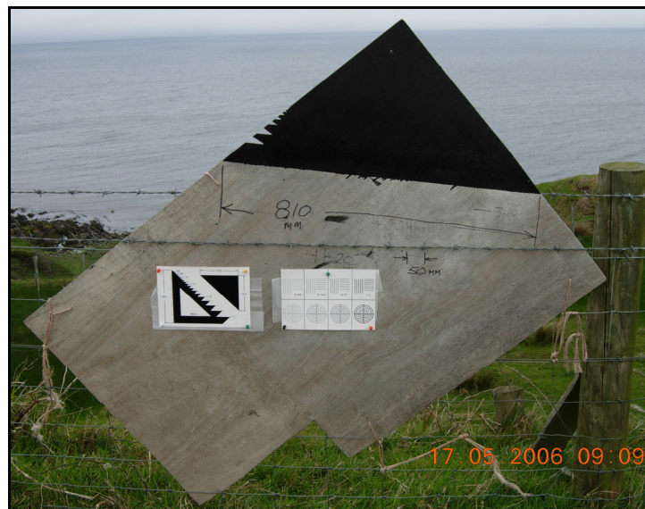
Figure 2.5: Land target used to test the digiscope. The width of the bottom of the black triangle is 81cm. Note that this image was taken using the camera only, not the assembled digiscope.
