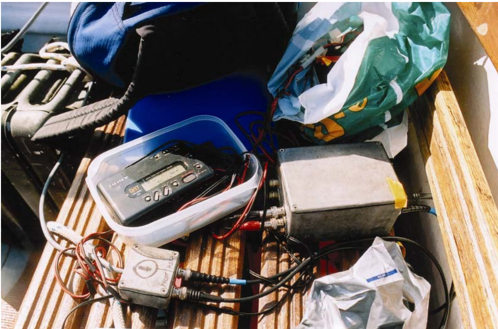
Figure 2.6. Hydrophone cables, high pass filter (on the right) and DAT recorder (top left).
