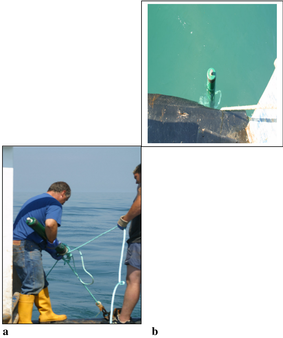
Figure 2.7. T-POD deployment from fishing boat. a. The anchor and preceding rope in the water and the T-POD and weight are ready to be deployed. b. T-POD on the way to the bottom.
