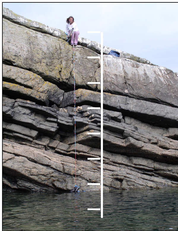
Figure 2.14. Measurement of tide height, with marked rope hanging from the TRF; and calibration of reticules (shown in white) from the reticulated binoculars, at New Quay.
