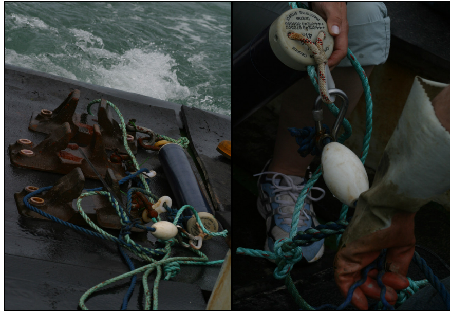
Figure 2.5. a. Picture of Mwnt T-POD mooring, note that a weight was used instead of an anchor. b. Picture showing the T-POD attachment to the mooring by a carabiner hook and an extra rope passing through T-POD lid. (Developed in cooperation with the fishermen; W. Evans and L. Walters)
