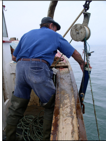
a b Figure 2.8. T-POD retrieving from fishing boat. a. Mooring ready to retrieved, rope caught with a hook. b. Mooring being pulled up with the winch and the T-POD is hanging on the side of the boat.
