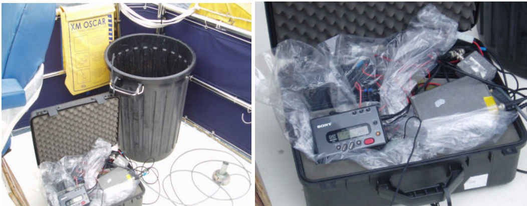
Figure 2.4 Figure; a) Hydrophone cables connected to the recording equipment. Figure; b) DAT recorder (left) and high pass filter (right)
