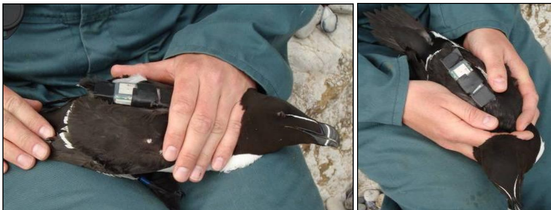
Figure 2.3 Modified I-got-U 120 GPS logger attached to the back feathers of a razorbill Alca torda . Photographs by Steve Dodd.
